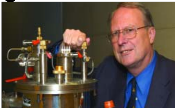
Seminal research: Jim Hough with a cryostat for the testing of cooled silicon as a test mass material for future gravitational-wave detectors.
